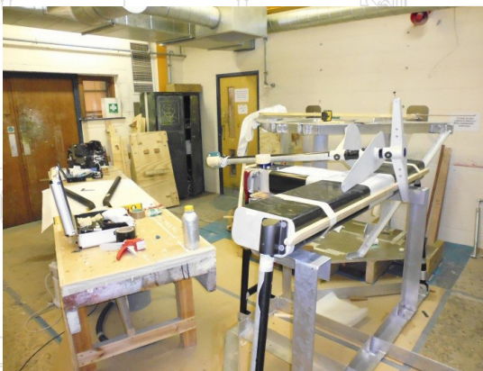
SHANNON MAST ASSEMBLY IN ITS JIG
