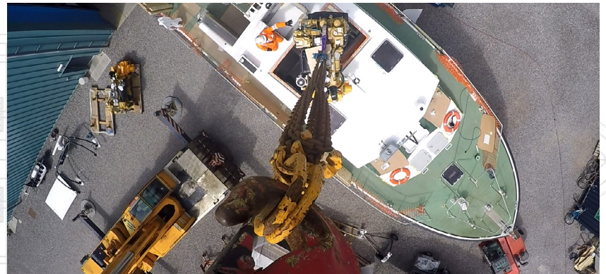
INSTALLING TWIN CATERPILLAR C18 810HP ENGINES
