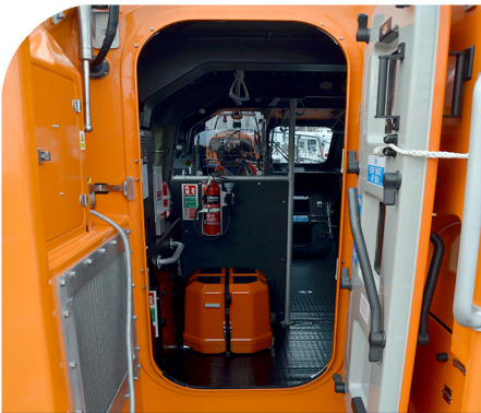
PROTECTED WHEELHOUSE ENTRANCE
