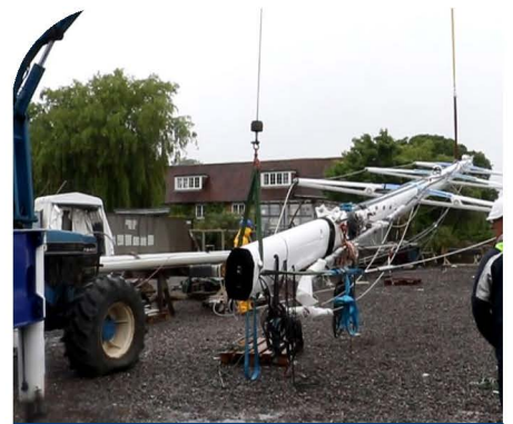
STEPPING THE NEW MAST
