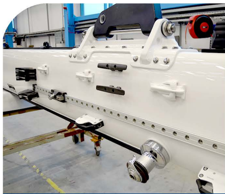
NEW MAST FITTINGS
