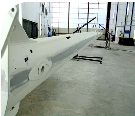
STRIPPED AND SANDED MAST
