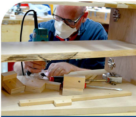
FABRICATING NEW CABINETS
