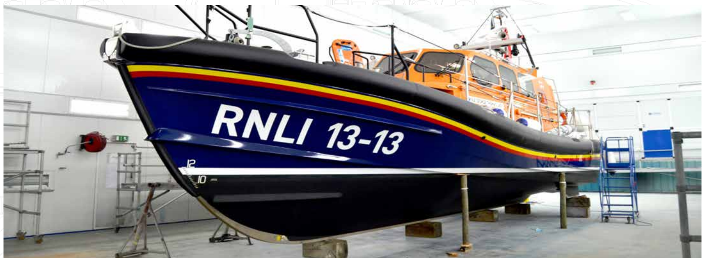
(6) POST-CURE BONDING OF THE HULL AND DECK TOGETHER IN BERTHON'S PAINT OVEN
