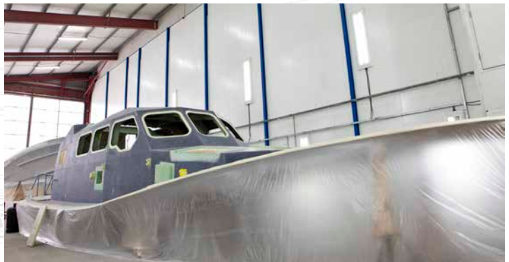
(3) DECK & WHEELHOUSE MOULD READY FOR PAINTING
