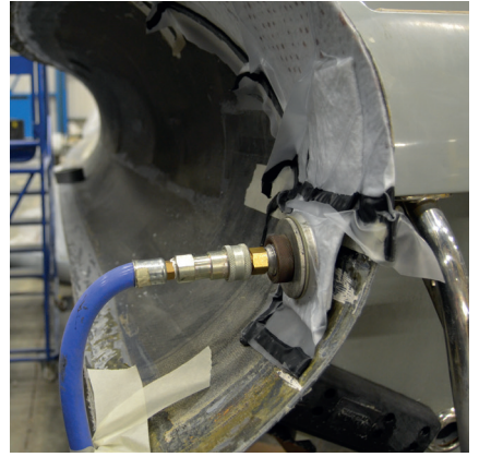
Structural repair to tube
