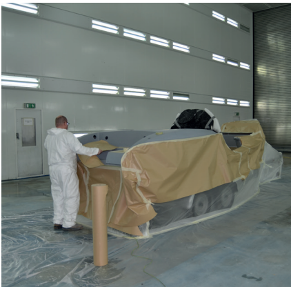
Preparation for painting
