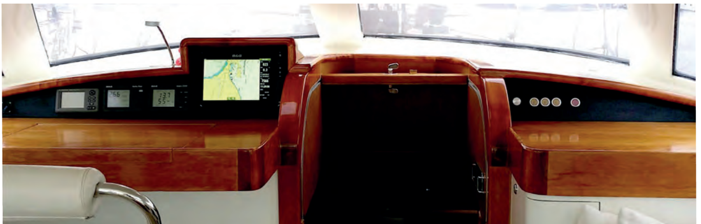
B&G Sailing instruments in the dog house
