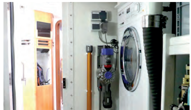
New washing machine fitted in lazarette
