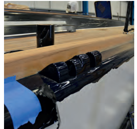
Refurbished chainplate mounts
