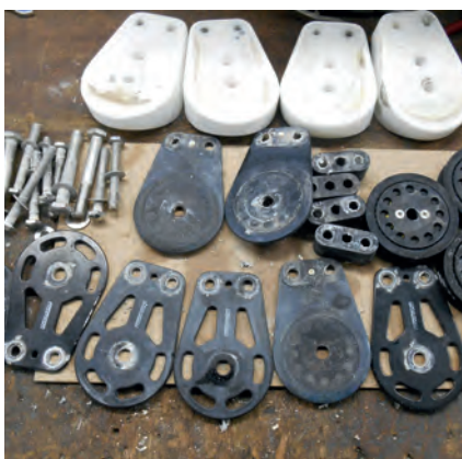
Stripped deck blocks and gears
