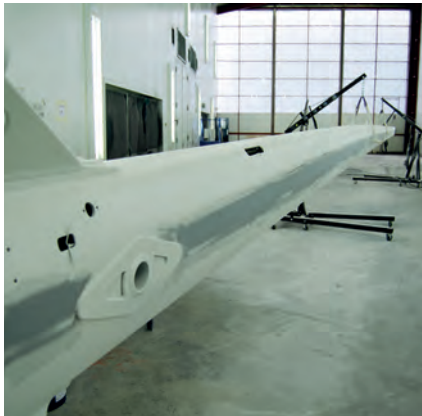
Stripped and sanded mast
