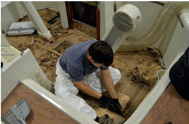
Removing the old teak deck
