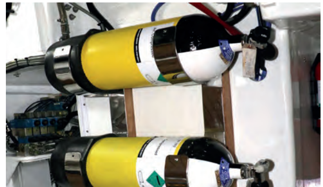
Custom racking for heavy dive equipment
