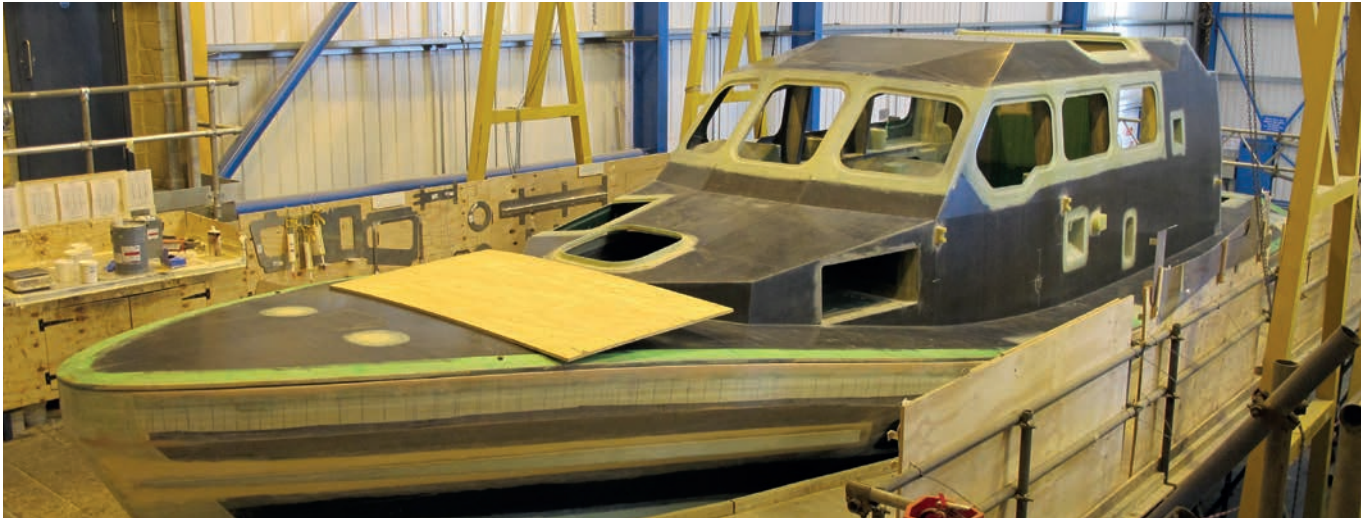
1 Hull and deck moulding 'trial fit'
