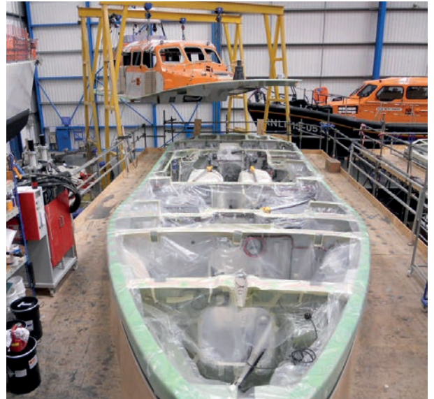
5 Deck and wheelhouse lifted onto the hull
