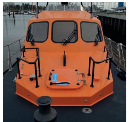
Heavily reinforced coach roof
