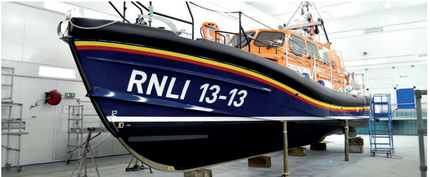
6 Post-cure bonding of the hull and deck together in Berthon's paint oven
