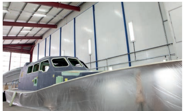
3 Deck and Wheelhouse mould ready for painting
