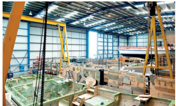
2 'Open-sky' composite fit out of hull
