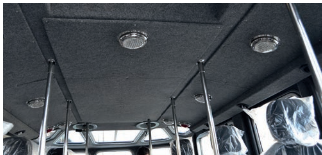
Insulated deckhead panels
