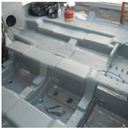
Engine bay ready for engines
