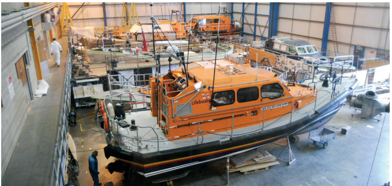
Production line of RNLI Shannon Lifeboats in one of our work sheds
