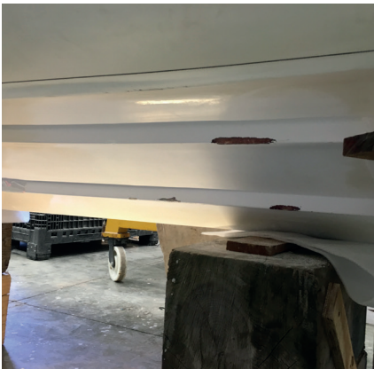
Hull damage After Beaching
