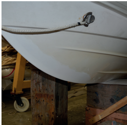
gelcoat showing repairs
