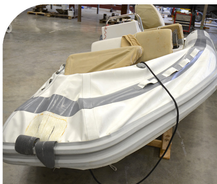
TUBE DAMAGE TO THE BOW
