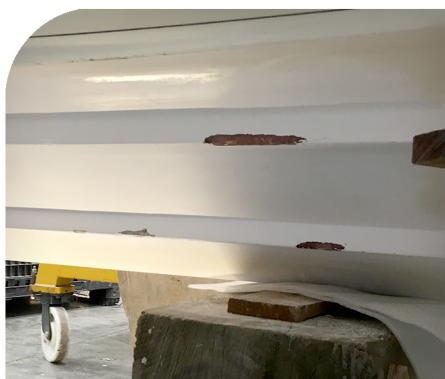
HULL DAMAGE AFTER BEACHING
