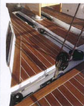
▲ Above: The single-point mainsheet traveller is a neat solution – the rams and workings are hidden under deck plates (exposed in this photograph)
