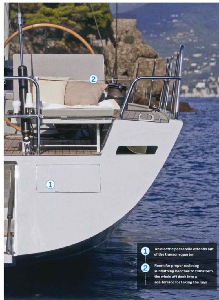
3 Aft deck transformation: a platform folds down and steps revolve inside to allow guests to walk down to the water's edge, swim and take a shower. Inside is a huge (2.8m) lazarette
