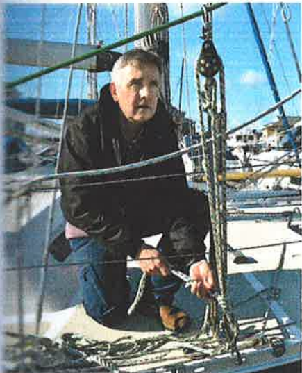
Adjust the angle of your spinnaker guy by using the handy-billy as a makeshift 'tweaker'
