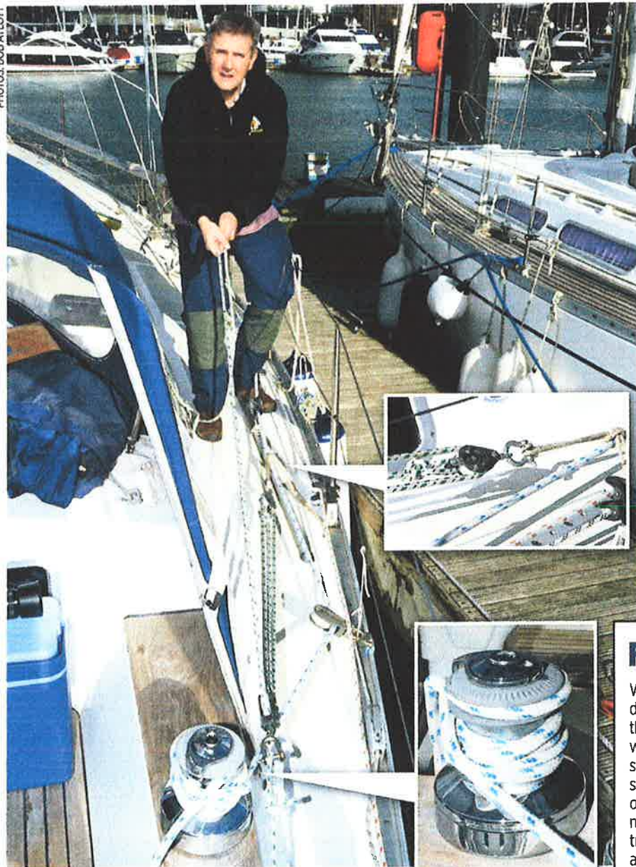
A riding turn can be serious in a squall. One way of freeing it is to take up the tension of the sheet with the handy-billy
