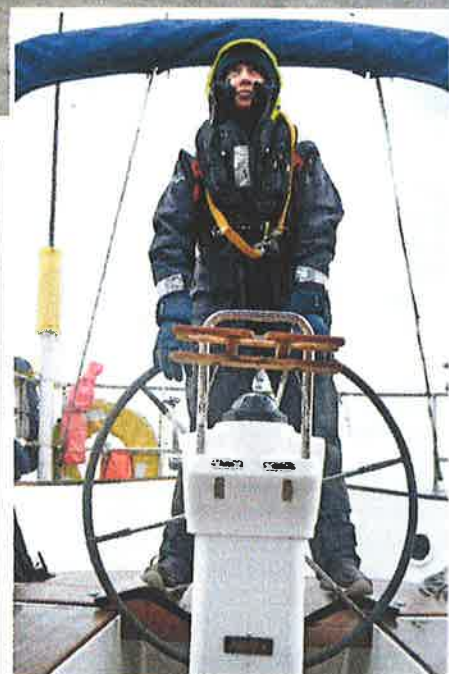
John used his own DIY skills to make this foot stand which gives the helm a view forward
